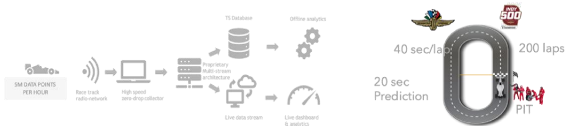
1 IndyCar telemetry configuration and lap distance
